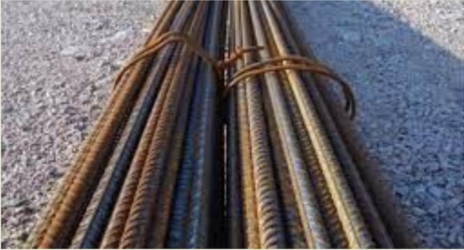
Using higher strength rebar to reduce the amount of rebar used
