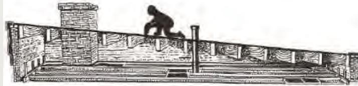
Inspect for roof leaks and weak ceilings. Note bypass locations from below (duct chases, closets, ceiling height changes, etc.). Cut an access hole big enough for a person but small enough for a foot vent.
