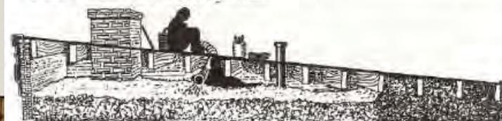
After all bypasses have been sealed, insulation blowing can be completed by one crawler. Be sure to allow for settling—read the bag and check your work with a bag course.
