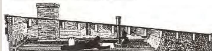
After dense packing is done, both crawlers continue to seal bypasses. Here, front crawler is installing drop-ceiling pipe while rear crawler is forming plumbing stack bypass.
