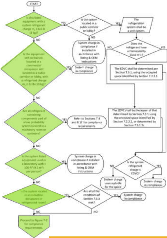
Figure 7-1 Refrigerant system charge limit compliance path—Part 1.
