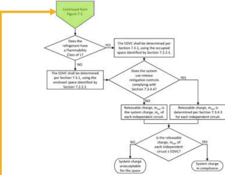
Figure 7-2 Refrigerant system charge limit compliance path—Part 2.
