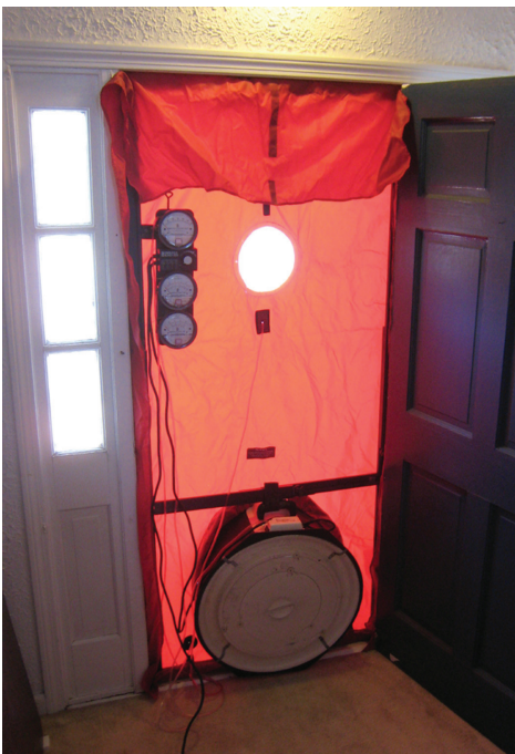
The blower-door setup at the Livermore home.
