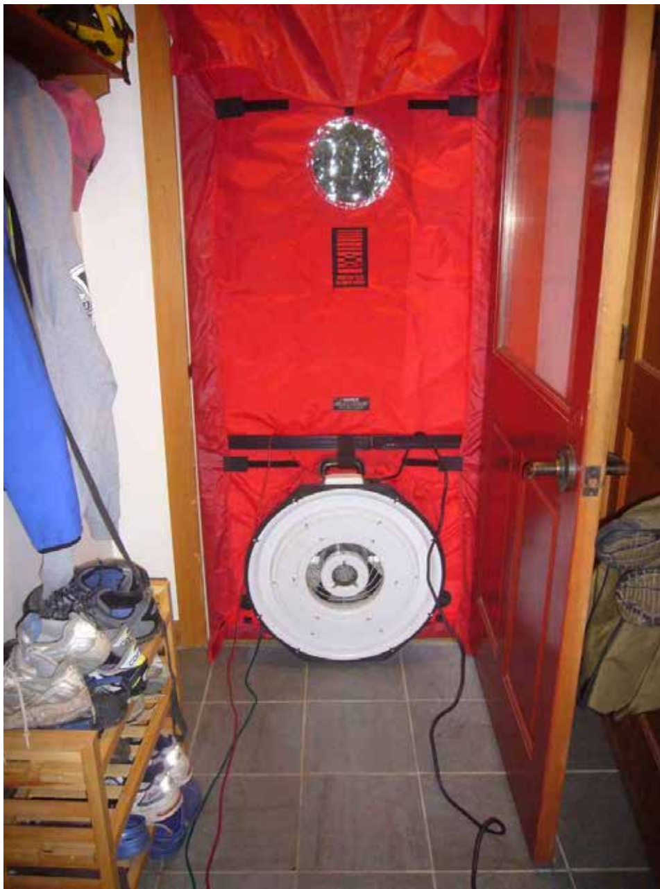
The tightest net zero homes are coming in at below 100 CFM50 on blower-door tests, compelling testers to invest in C-, D-, and even E-rings (shown here).
