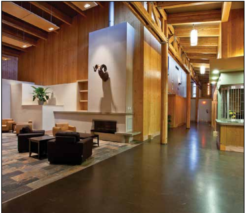
CrossLam is a cross-laminated timber (CLT) structural panel that can be used for floors, walls, and roofing. CLT is made from less desirable wood, including wood taken from forests killed by mountain pine beetles, but higher-quality wood can be used if it is going to be exposed to view.
