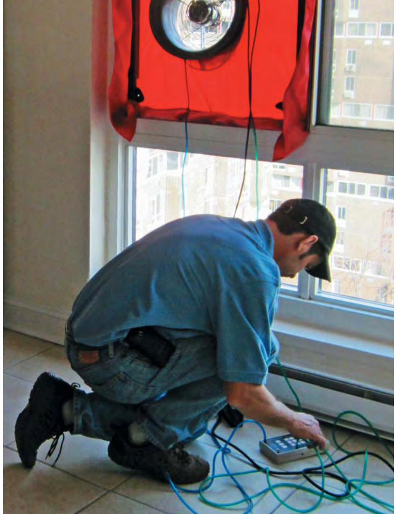
A CREW MEMBER PERFORMS AN AIRFLOW TEST AT THE ROOSEVELT LANDINGS COMPLEX ON FEB. 22, 2012.
