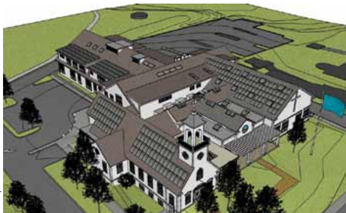
Sketch-up model showing proposed photovoltaic system arrays.
