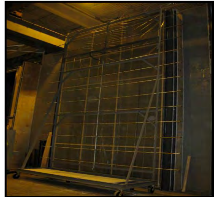
Photo No. 1 Exterior View during Air Infiltration Test
