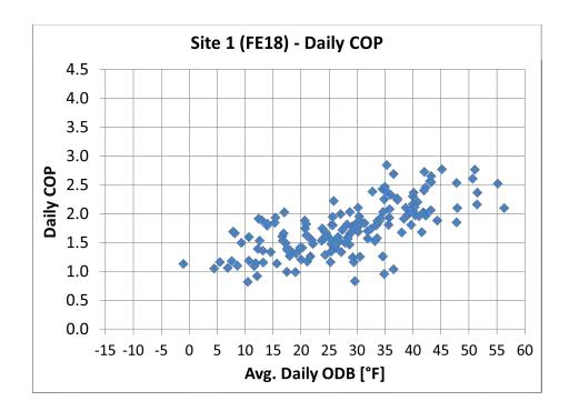
High return air temperatures lead to lower heating efficiencies, so...
