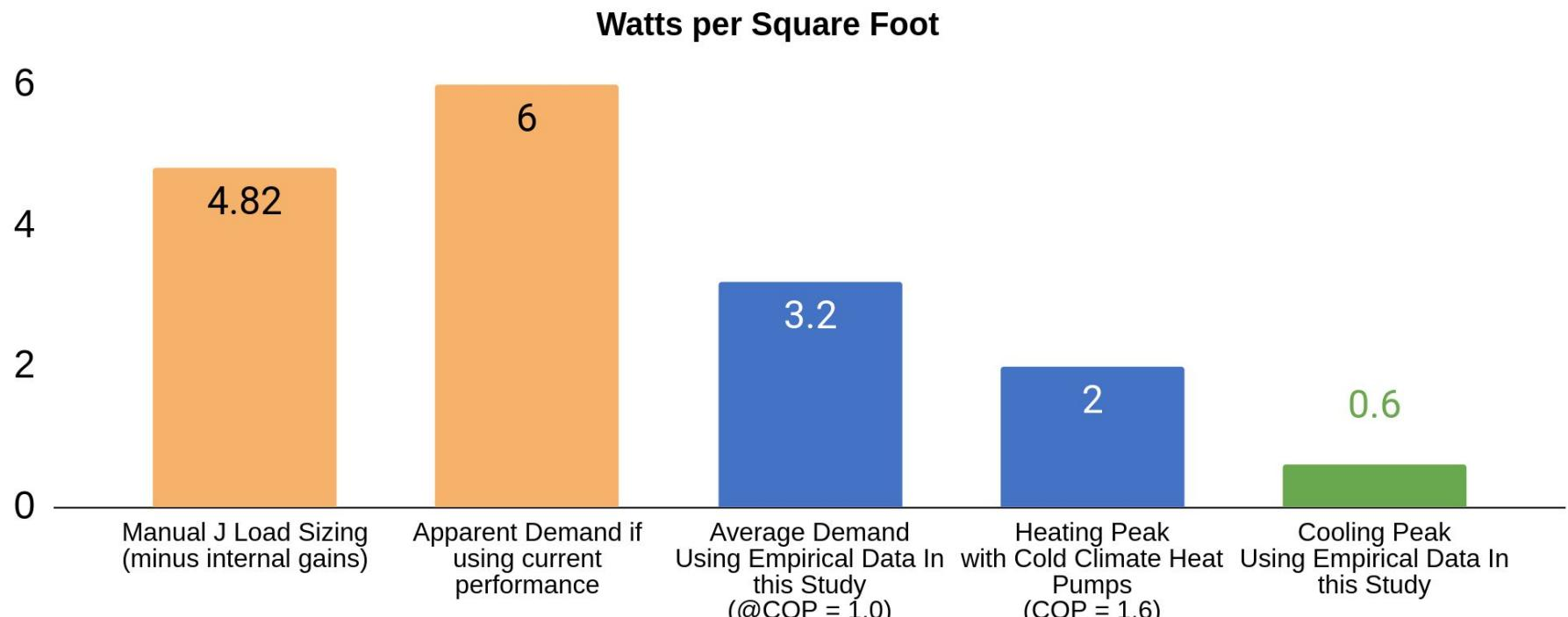
\*Watts/SF of apparent heating demand = Typical Fossil Fuel Heat slope \* boiler efficiency \* 60 HDD / 24 Hours / 3.412btu/W
