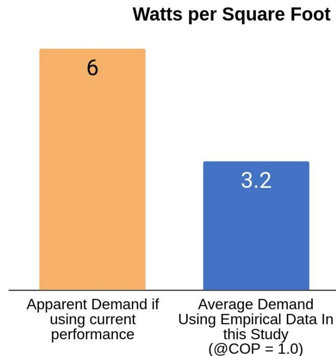
\*Watts/SF of apparent heating demand = Typical Fossil Fuel Heat slope \* boiler efficiency \* 60 HDD / 24 Hours / 3.412Btu/W
