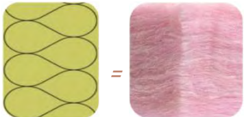
Existing fiberglass batt insulation
