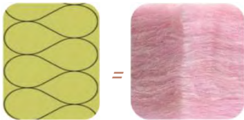
Existing fiberglass batt insulation
