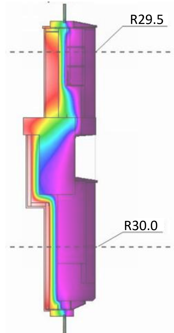
Interior Insulation 3 1/2" Spay Foam
