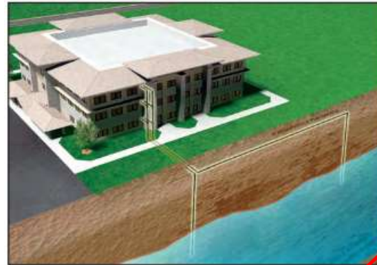
Open loop, "pump and dump"
