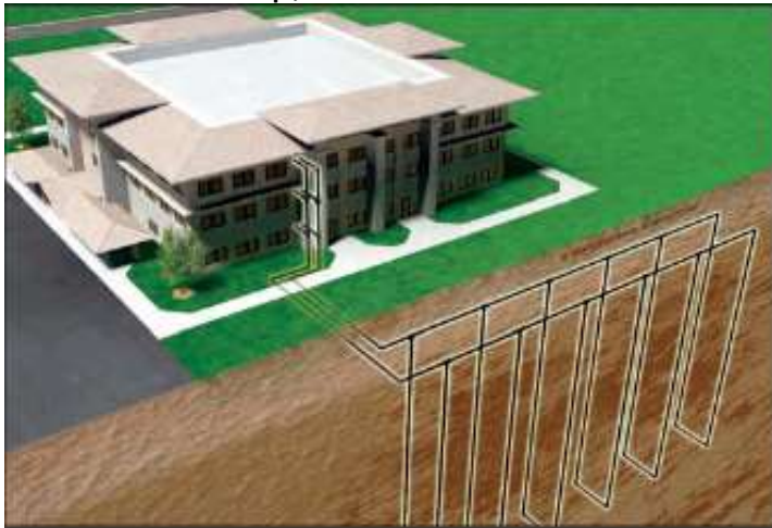
Closed loop, boreholes
