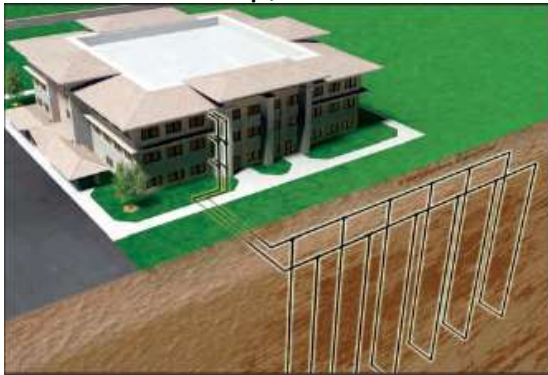
Closed loop, boreholes
