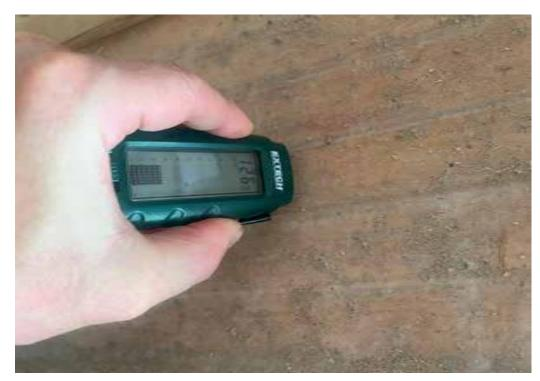
Doug Fir <19M% when delivered (as code requires) – it was 15M% Protection with transparent membrane – semi vapor permeable – PROTECT keep dry from rain and allows drying to 12M% in few months
