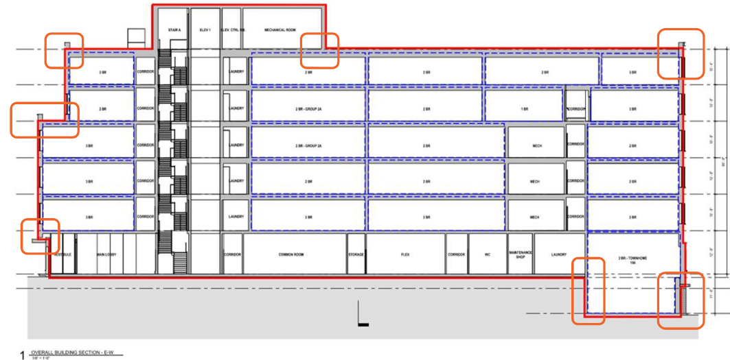
1 OVERALL BUILDING SECTION - E-W 1" = 10'-0"
